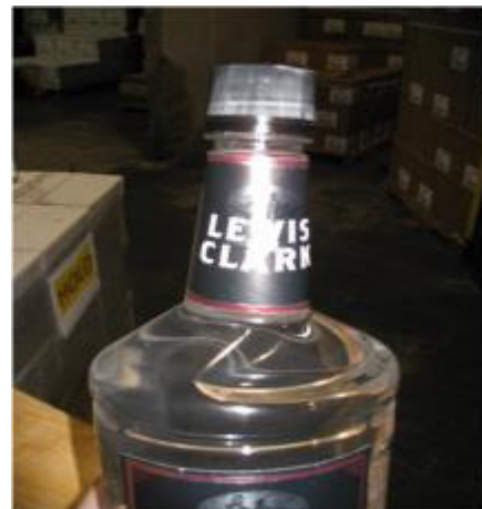
The buckling shown here is one of the many failure modes of lightweight plastic packaging, something that Amcor has helped eliminate using SIMULIA’s simulation software.
