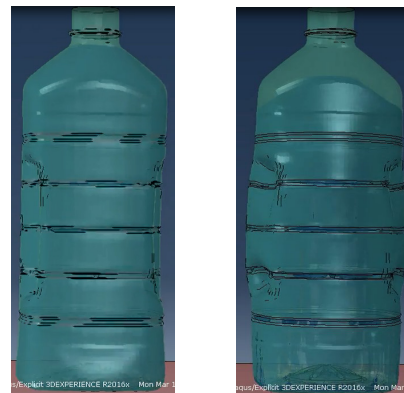
Simulation of container bulging when dropped.
