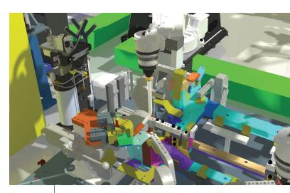
**Top image:** Simulation allows CenterLine to transfer robot system programs to the factory floor and the robot without tying up physical resources on the floor.
