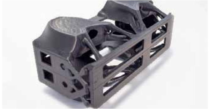
Figure 3a: Topology optimized circuit box for space rocket.
